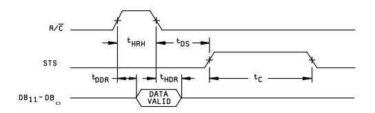
HIGH PULSE FOR R/C - OUTPUTS ENABLED WHILE
