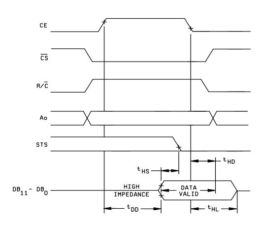
FIGURE 6. Read cycle timing.
