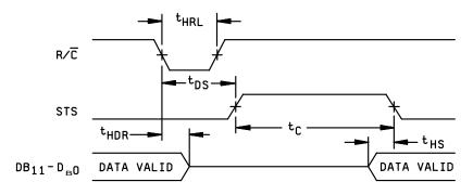
LOW PULSE FOR R/C - OUTPUTS ENABLED
