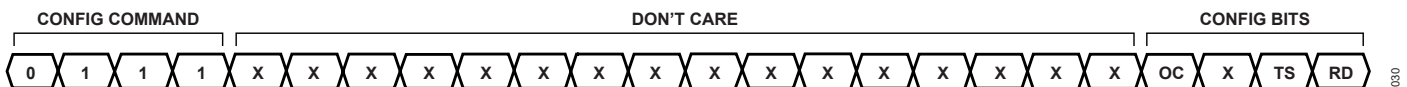
Figure 33. Configuration Command Syntax, Open-Circuit (OC) Detection Disable, Thermal Shutdown (TS) Disable, and Reference Disable (RD)
