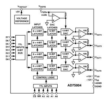
The bandgap reference on the chip has low noise, long term stability and temperature drift characteristics comparable to discrete reference diodes. The absolute value of the reference is laser trimmed to +5.00 V with 0.6% maximum error. Its temperature coefficient is also laser trimmed.
