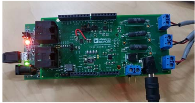
Figure 9. EVAL-CN0410-ARDZ Evaluation System
