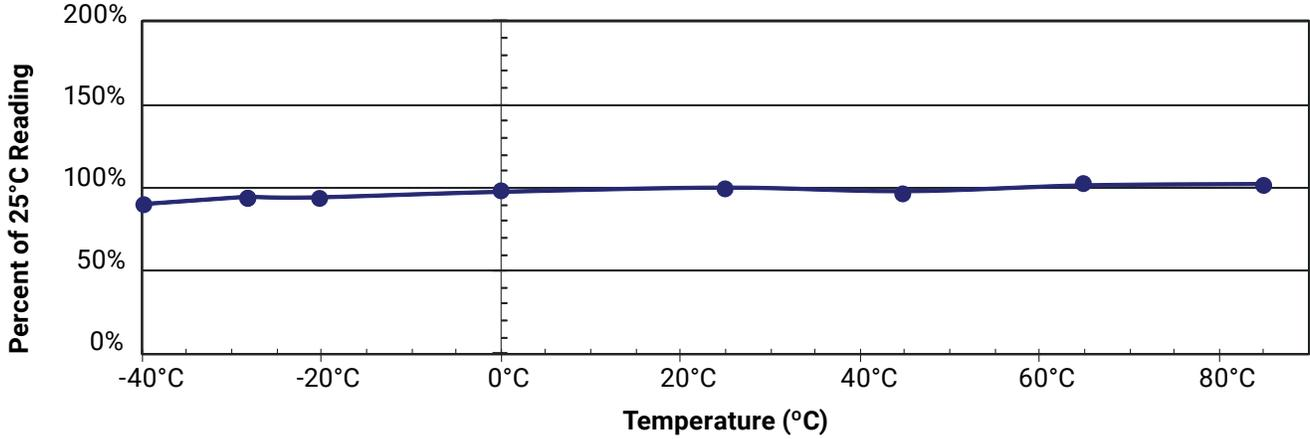
LEAKAGE CURRENT VS. TEMPERATURE
