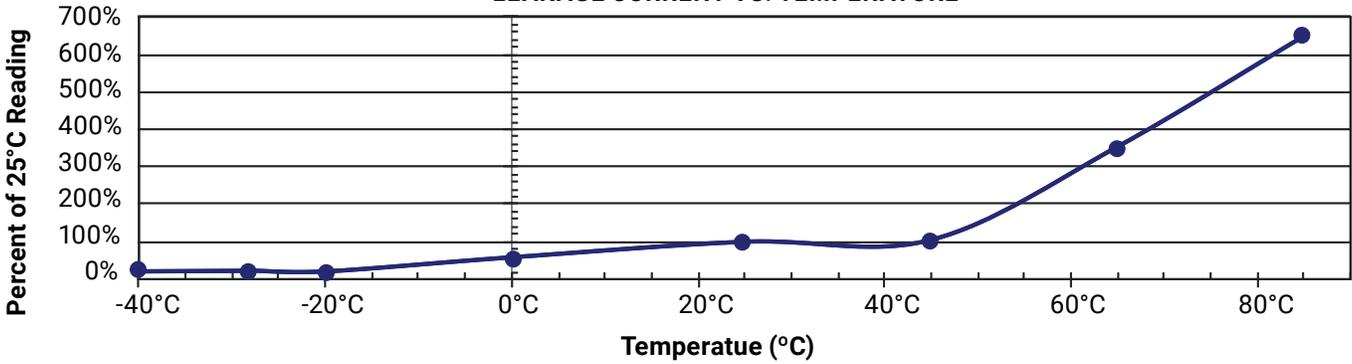
EQUIVALENT SERIES RESISTANCE VS. TEMPERATURE
