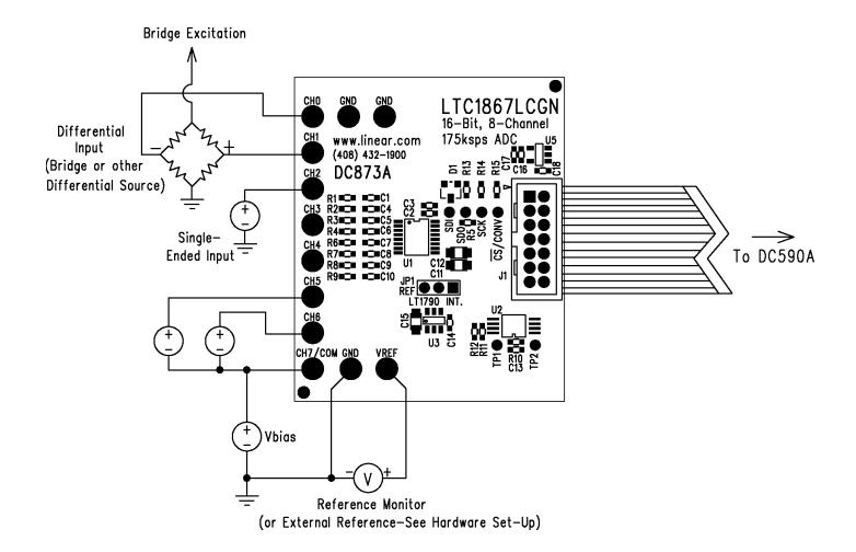
Figure 1. Connection Diagram
