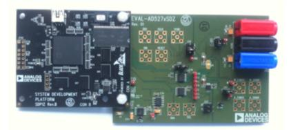
The **EVAL-AD5270SDZ** evaluation board is a member of a growing number of boards available for the **SDP**. Designed to help customers evaluate performance or quickly prototype new **AD5270** circuits and reduce design time, the **EVAL-AD5270SDZ** evaluation board can operate in single-supply and dual-supply mode and incorporates an internal power supply powered from the USB.
