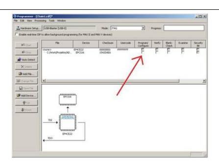
After finishing, the image is permanently loaded to the configuration Flash and the system will start with a blinking LED after reset or power up.
