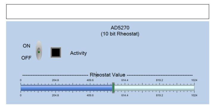
The communication with the board is activated / deactivated by toggling the **ON/OFF** switch. The **Activity** LED turns green when the communication is active. If the **ON/OFF** switch is set to **ON** and the **Activity** LED is **BLACK** it means that there is a communication problem with the board. See the **Troubleshooting** section for indications on how to fix the communication problems.
