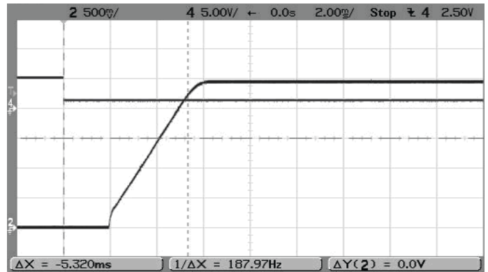
Step Load Transient Response (Vin=5V, Vout=2.5V, Clod=0, Iout=3A to 1.5A) Trace 2=Vout, 100 mV/div. Trace 4=Iout, 2.5A/div.
