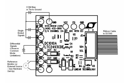
Figure 1. Proper Measurement Equipment Setup
