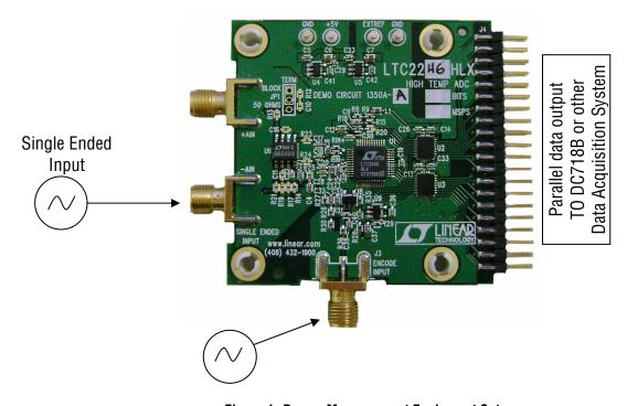
Figure 1. Proper Measurement Equipment Setup
