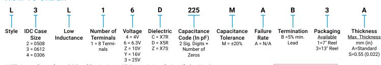
NOTE: Contact factory for availability of Termination and Tolerance Options for Specific Part Numbers.
