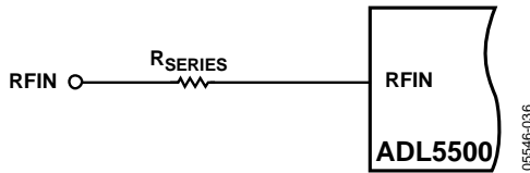
Figure 36. Attenuating the Input Signal
