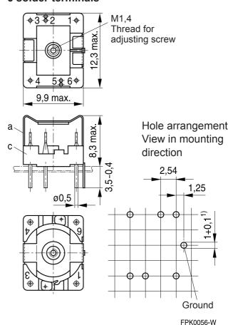
b) Terminal carrier with 4 solder terminals
