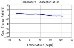
GCJ216R72A682KA01 C-Temp. capchange, DCO.OV, AC1.C
