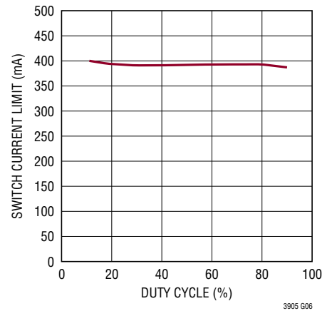
Switch Current Limit vs Duty Cycle
