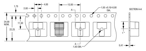
TOLERANCES: ±0.13 UNLESS OTHERWISE SPECIFIED **DIMENSIONS: MILLIMETERS**
