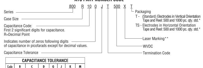
The above part number refers to a 800 R Series (case size R) 10 pF capacitor, J tolerance (±5%), 500 WVDC, with T termination (Tin Plated over Nickel Barrier, RoHS Compliant), laser marked, and tape and reel packaging. \*Consult ATC for other quantities. \*\*Laser Marking is optional.
