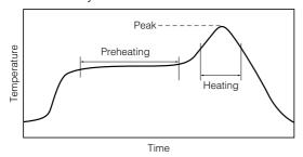
For soldering (Example : Sn/Pb)
