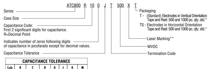
The above part number refers to a 800 R Series (case size R) 10 pF capacitor, J tolerance (±5%), 500 WVDC, with T termination (Tin Plated over Nickel Barrier, RoHS Compliant), laser marked, and tape and reel packaging.
