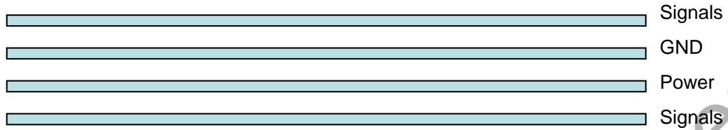
Figure 29: Typical 4-layer PCB construction
