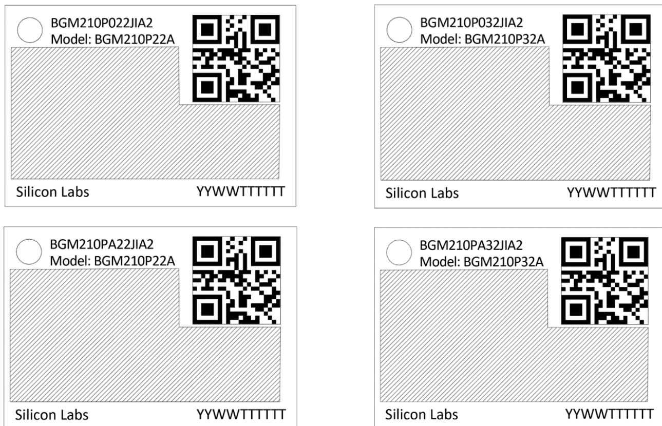
Figure 8.4. BGM210P Top Marking
