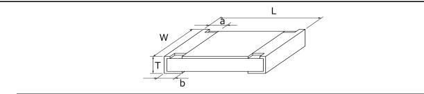
Mass Part No. **Dimensions** (Weight) (inch size) W b (g/1000 pcs) а EZAEG1N  $0.15 \pm 0.10$  $0.60 \pm 0.03$  $0.30 \pm 0.03$  $0.15 \pm 0.10$  $0.23 \pm 0.03$ 0.12 (0201)EZAEG2N  $1.00\pm0.10$  $0.50 \pm 0.05$  $0.20 \pm 0.10$ 0.27±0.10  $0.38 \pm 0.05$ 0.60 (0402)
