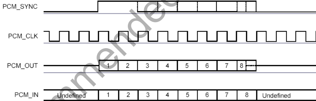
Figure 18: Long Frame Sync (Shown with 8-bit Companded Sample)
