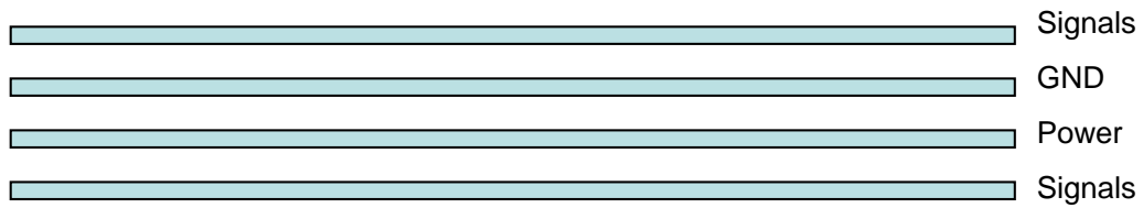
Figure 29: Typical 4-layer PCB construction
