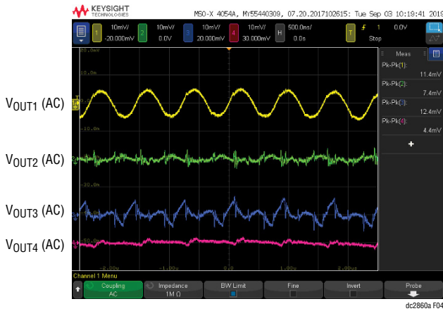
Figure 4. Output Voltage Ripples
