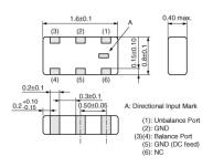
\*Terminal of \*NC" should be fixed to the no connected pattern.
