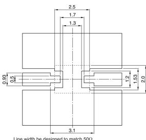
Line width be designed to match  $50\Omega$  characteristic impedance depending on PCB material and thickness.
