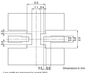
Line width be designed to match  $50\Omega$  characteristic impedance depending on PCB material and thickness.
