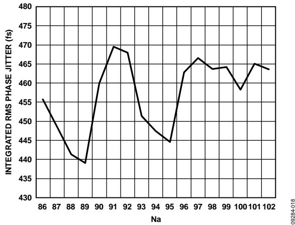
Figure 18. Typical Integrated Random Phase Jitter in fs rms for PLL1 and OUT0P LVPECL as Feedback Divider Value Na Swept ( f_{XTAL} = 25 MHz, V0 = 5 , D0 = 5 )
