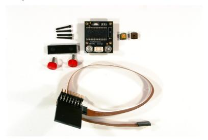
ICE Debugging Support for QFN CY8C21x34 PSoC Devices in a Prototype System or PCB
