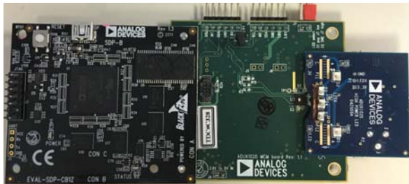
Figure 9. Connecting the ADUX1020-EVALZ-LED Daughterboard
