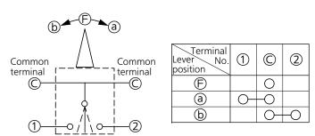
Note) Contact and Insulation on close not apply on between frame and common terminal.
