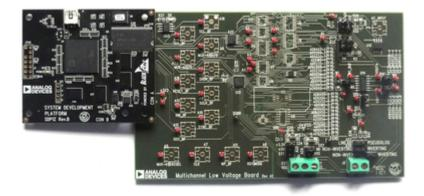
The EVAL-AD5162SDZ evaluation board is a member of a growing number of boards available for the SDP. Designed to help customers evaluate performance or quickly prototype new AD5162 circuits and reduce design time, the EVAL-AD5162SDZ evaluation board can operate in single-supply and incorporates an internal power supply powered from the USB.
