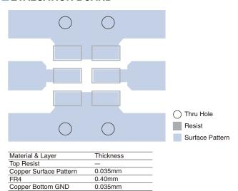
Line width should be designed to match  $50\Omega$  characteristic impedance, depending on PCB material and thickness.
