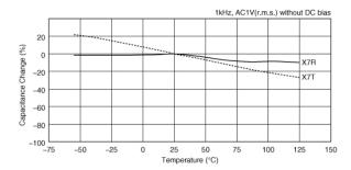
Capacitance - temperature characteristics
