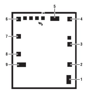
61mils × 72mils, 12mils thick. †Backside metal: Alloyed gold layer (K designator) Backside potential: lowest (GND) voltage
