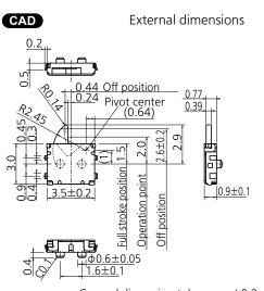
General dimension tolerance: ±0.3 PWB mounting hole for reference
