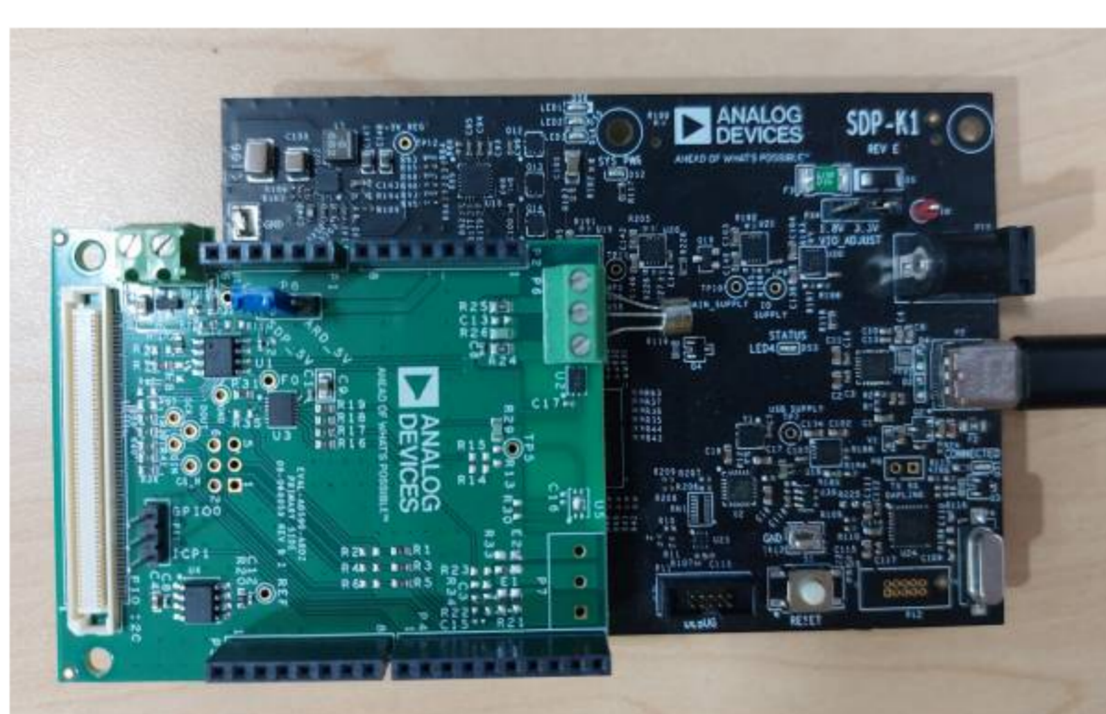
Figure 3. EVAL-AD590-ARDZ BOARD AND SDP BOARD CONNECTED DIAGRAM
