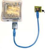
**NOTE:** A flex-pod is a flex-cable with an emulation chip on the cable.
