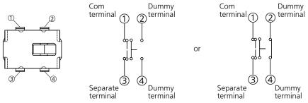
Note) Contact and Insulation on close not apply on between cover and dummy terminal.
