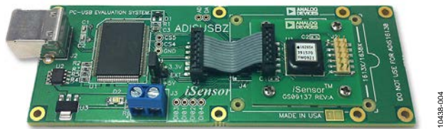
Figure 3. ADIS16265/PCBZ and ADISUSBZ
