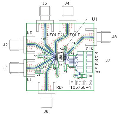
The circuit board used in the final application should use RF circuit design techniques. Signal lines should have 50 ohm impedance while the package ground leads and backside ground slug should be connected directly to the ground plane similar to that shown. A sufficient number of via holes should be used to connect the top and bottom ground planes. The evaluation circuit board shown is available from Hittite upon request.
