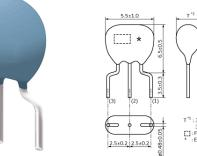
T<sup>11</sup>: 3.5±1.0 (16.00–32.99MHz) 3.0±1.0 (33.00–70.00MHz) : Frequency Marking \* : EIAJ Monthly Code (in mm) Features
