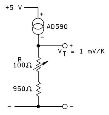
NOTE: V<sub>S</sub> across device must remain constant or PSRR error must be included.
