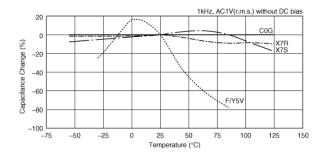
Capacitance - temperature characteristics
