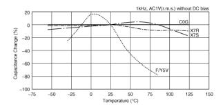
Capacitance - temperature characteristics
