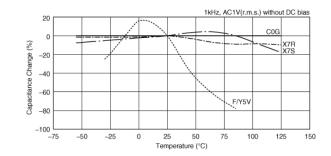
Capacitance - temperature characteristics
