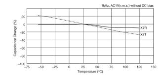
Capacitance - temperature characteristics
