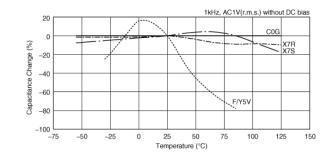
Capacitance - temperature characteristics
