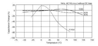
Capacitance - temperature characteristics
