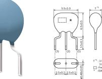
T<sup>11</sup>: 3.5±1.0 (16.00–32.99MHz) 3.0±1.0 (33.00–70.00MHz) : Frequency Marking \* : EIAJ Monthly Code (in mm) Note: This datasheet may be out of date. Please download the latest datasheet of CSTLS16M0X51-B0 from the official website of Murata Manufacturing Co., Ltd.
